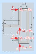
In the figure above, the dashed lines indicate the lever arms of the forces. Based on these distances, we obtain the moments.
