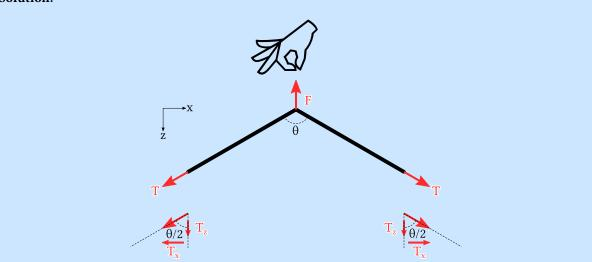
We introduce a coordinate system and decompose T into its x- and z-components  $T_x$  and  $T_z$ , respectively. From geometry  $T_x = \sin(\theta/2)T$  and  $T_z = \cos(\theta/2)T$ . For the system to be in equilibrium, the force F must be balanced by the two components  $T_z$ , i.e.
