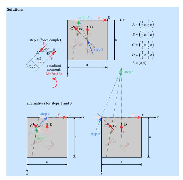
**step 1** The forces at A and B are equal and opposite. Therefore, their contribution to the resultant force is zero. However, they create a positive (counter-clockwise) moment about the y-axis (pointing out of the plane of the paper). The distance between the lines of actions is  $a/(2\sqrt{2})$ , therefore the magnitude of the moment is  $M = Fa/(2\sqrt{2})$ .
