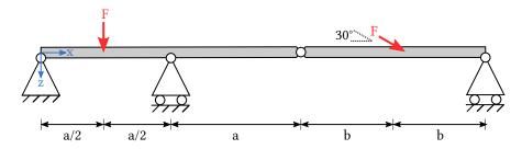
**Solution:**  $n=2, r=4, v=2, \quad 3\times 2-(4+2)=0 \implies$  the structure is statically determinate. We will cut the girder at the hinge and require equilibrium for each of the two bars. Keep in mind that  $\sin(30^\circ)=1/2$  and  $\cos(30^\circ)=\sqrt{3}/2$ .
