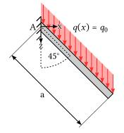
**Solution:** To find the resultant of the line load, we need to integrate along the length of the beam. For this purpose, we introduce a coordinate system whose x'-axis is aligned with the beam axis and split the line load into parallel and perpendicular components  $q_N(x')$  and  $q_Q(x')$ , respectively. Considering the angle, we obtain
